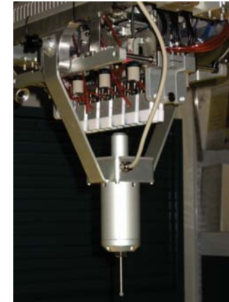
View of mechanical touch probe
